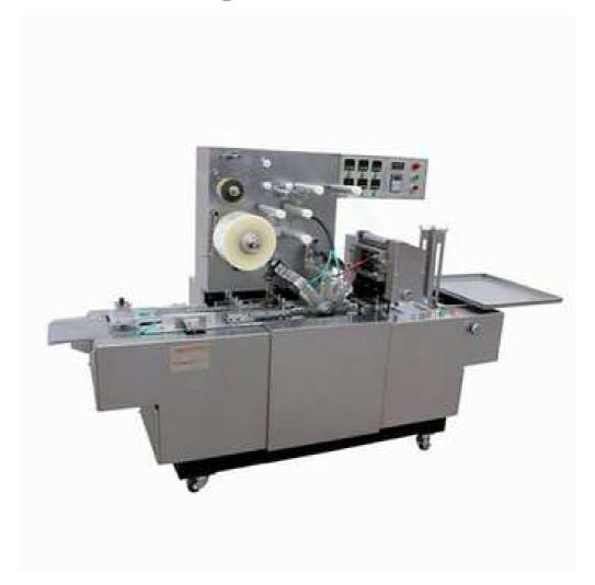
The packaging machine is a full-automatic three —dimensional packing machine. Made of materials including BOPP film and PVC, the machine can apply to wrapping the products as a folding hexahedral single-box package. It's an ideal for the cassette packing cases.
